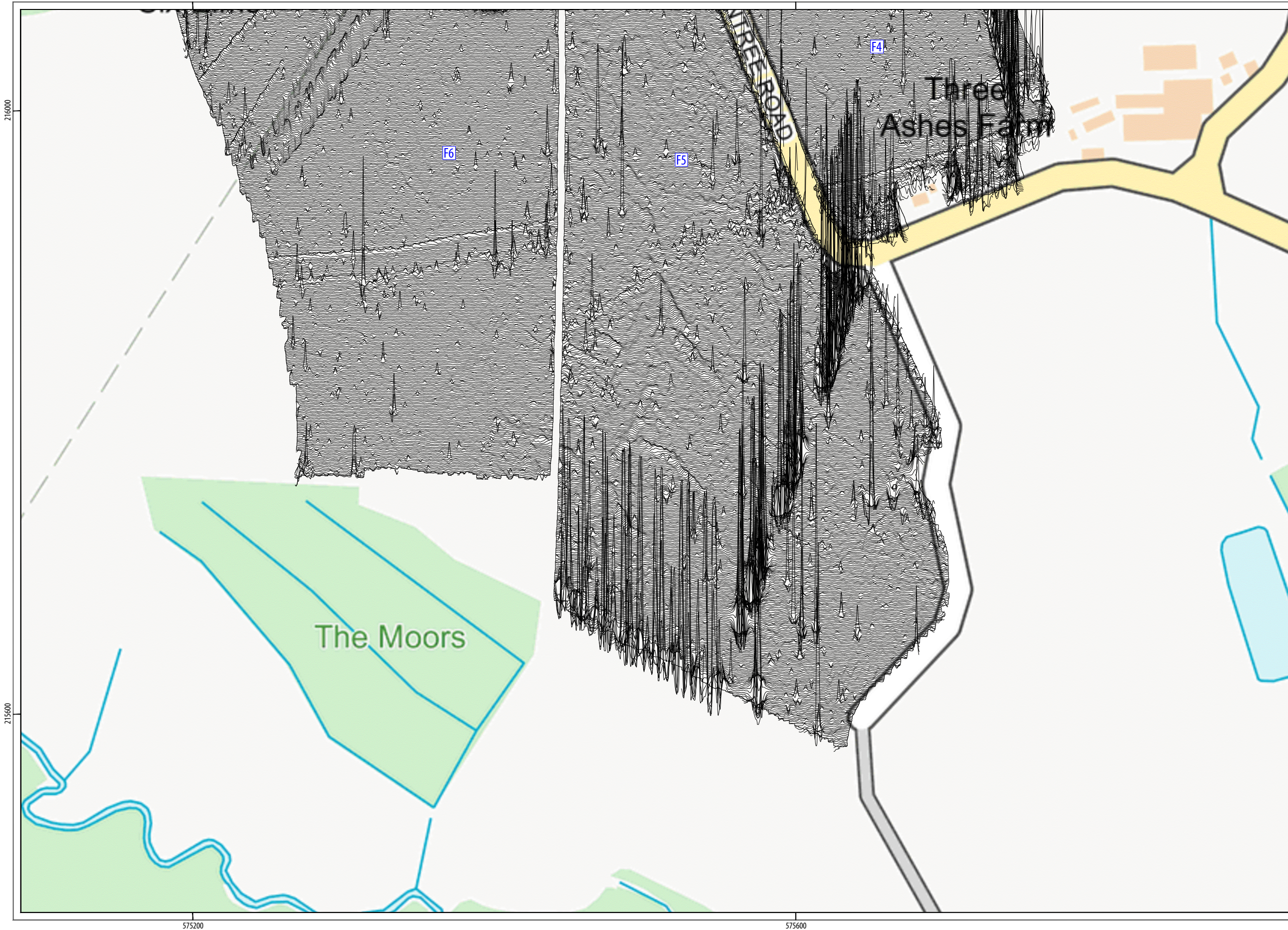
ILLUS 20 XY trace plot of minimally processed magnetometer data; Area 3
