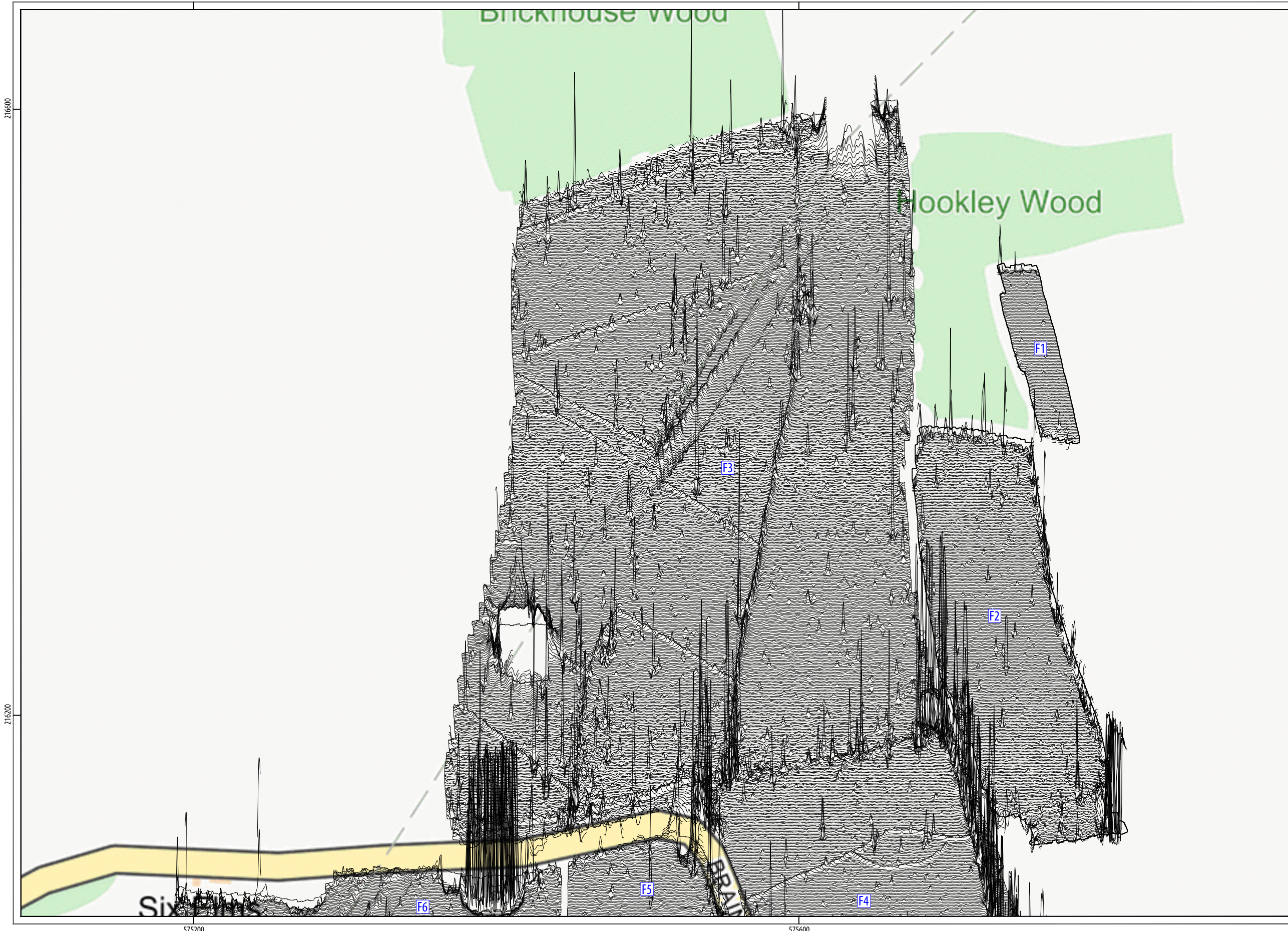
ILLUS 14 XY trace plot of minimally processed magnetometer data; Area 1
